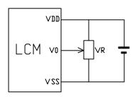
V<sub>DD~</sub>V<sub>0</sub>: LCD Driving voltage VR: 10k~20k
